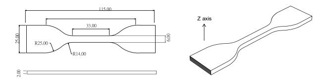
Tensile testing specimen; ISO 37
